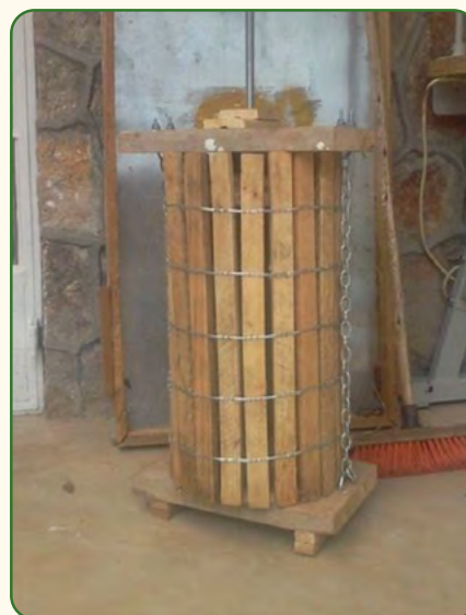
Image. A honey extraction bush press made from local materials.
